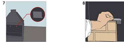
Fig. 7. Holder at the backside of the insert for fixing the back wall insulation. Fig. 8. Install the back wall. At the bottom, fix it behind the bottom panel and with the clamps at the top.
