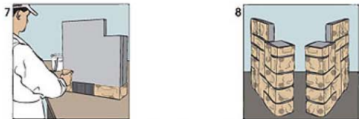
Fig. 7. Stick the facing on the Super-Isol boards using elastic glue. Fig. 8. The sidewalls made of Super-Isol boards need no additional insulation.
