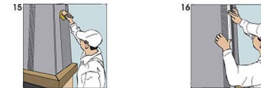
Fig. 15. Ground the exhaust duct cover. Fig. 16. Strengthen the board connections with joining tape and aluminium angles.
