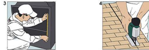
Fig. 3. Measure the insert and draw the cutting lines. Fig. 4. Cut the panels according to the measurements of the insert.
