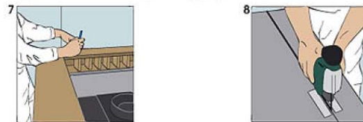
Fig. 7. Place the wooden girder and measure the required length of its insulation elements. Fig. 8. Cut out the required elements.
