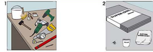
Fig. 1. Prepare the required tools. Fig. 2. Required material: Super-Isol board (30 mm recommended) SKAMOLEX Glue for joining, screws for wood (length = 2x used Super-Isol thickness, any elastic glue for attaching the Super-Isol boards to the wall behind the fireplace.
