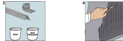
Fig. 3. Additional finishing materials: joining tape, aluminium angle with a net, grounding preparation, filling pulp. Fig. 4. Install the back wall, put the elastic glue on the board with a notched trowel.
