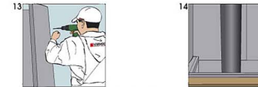
Fig. 13. After installing the sidewalls of the exhaust duct, stiffen the construction using the screws. Fig. 14. The chimney lead-out.
