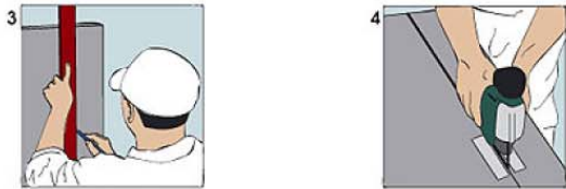
Fig. 3. Draw the cutting lines. Fig. 4. Cut out the elements of a sidewall with a jigsaw.
