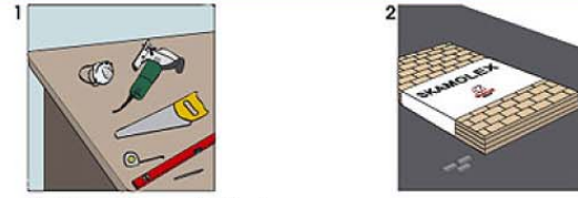
Fig. 1. Prepare the required tools. Fig. 2. Required material: SKAMOLEX heat-resistant panels, a set of installation clamps.
