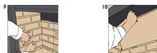
Fig. 9. Install the sidewalls. Fig. 10. Install the deflector. Lean it against the back wall and a steel peg.
