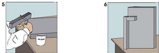
Fig. 5. Connect the element of the wall with the glue according to the instructions on the label. Fig. 6. Ground the construction before sticking to the facing.
